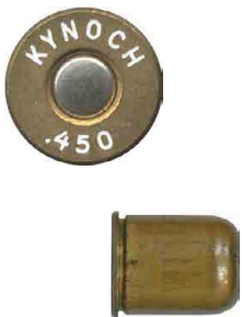
Blank: Brass case, nkl primer, undercut rim, open creased roll crimp over pink wad, o/a 0.606"
