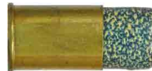
Shot: Brass case, brass primer, paper sabot with roll crimp over white wad.
