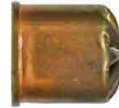
Blank: CW Brass case, brass primer, tight 8-point crimp, tan wad just visible, o/a 0.537". From M. Gaupillat tin shown above.
