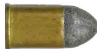
Proof: Brass case, copper primer, lead bullet. O/a wt.: 190 gr. Note differences in spelling, and case/bullet specifications compared to the factory drawing on page 114 of original book. .
