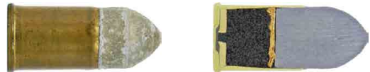
Ball: Brass case, brass primer flush with case head, 238gr. lead bullet.
