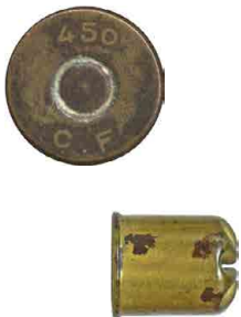
Blank: Brass case & primer, 6-pt open crimp over tan wad, o/a 0.599".
