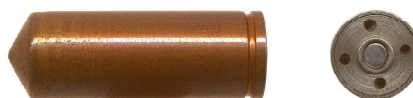
Fig. 12-3. Production .49-caliber (12.55 x 35.82mm) copper-plated steel Gyrojet with plain steel nozzle and nickel-plated primer cup. MBA's first production gyrojet. Actual size.
