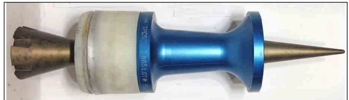
Photo 13a. Experimental M865 TPCSDS-T projectile with elongated sabot, fluted cone stabilizer and wide obturating band that snaps “into” the CCC adaptor. Not adopted for service.
