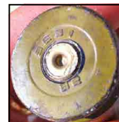
Photo 31/32 Chinese 14.5 × 114 mm BZT armour-piercing incendiary tracer (API-T) cartridge produced in 1972 by State Factory 631. © C.J. Chivers/The New York Times
