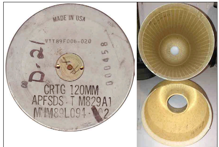
Photo 2c (right). Inside view of a combustable cartridge case (CCC) and its case adaptor constructed from cellulose.
