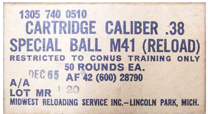
Figure 9. Reloaded ammunition was issued at one time for training as an economy measure as can be seen from this box dated 1965. This ammunition proved to be unsatisfactory in the field and most of it had to be destroyed.
