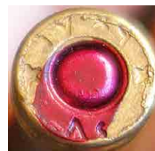
Photo 44 Syrian 9 × 18 mm cartridge produced in 1984 by the Industrial Establishment of Defence (EID). Note Arabic characters reading ‘9 × 17’. © C.J. Chivers/The New York Times
