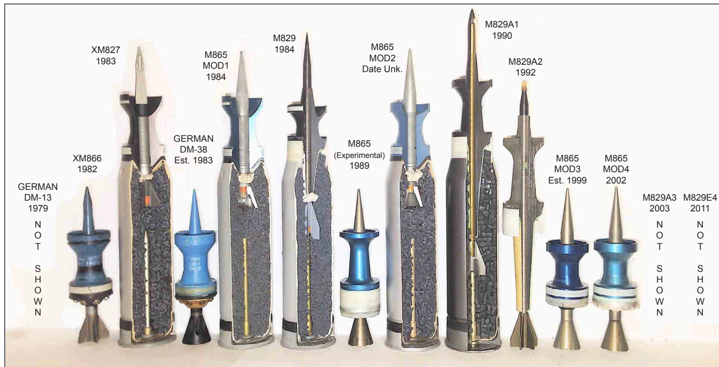
Photo 1. Complete developmental timeline sequence of US-made, 120mm tank-fired, APFSDS-T, TPFSDS-T & TPCSDS-T ammunition adopted for use in the Abrams M1A1 & A2 MBT’s
