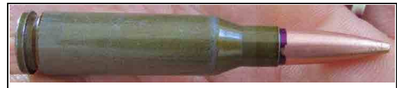
Photo 41 Russian 5.45 × 39 mm FMJ cartridge produced in 1998 by Barnaul Machine Tool Plant JSC. © Damien Spleeters
