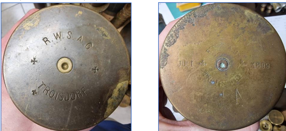
Figure 4: Left a 4-pointed “snow flake” on a 53x175R64 (5,3 cm Gruson) with a Swiss acceptance mark (“+”) and right an alternative “flaming bomb” on a 1899 dated 78x100R91 (blank for 7,7 cm FK96 nA, the additional “A” on the shell case is for “Ausschuss” (reject)). Clearly a “copy” of the Lorenz and DWM marks.
