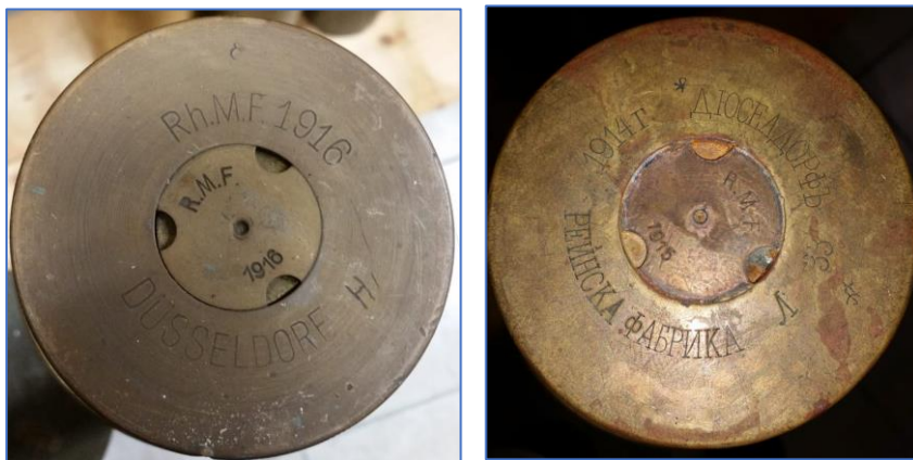
Figure 9: Left a 1916 dated RhMF shell case for export with a typical RhMF primer marked “R.M.F. 1916”, right a 1914 dated export shell case for Bulgaria with lot (not shell case) number 33.
