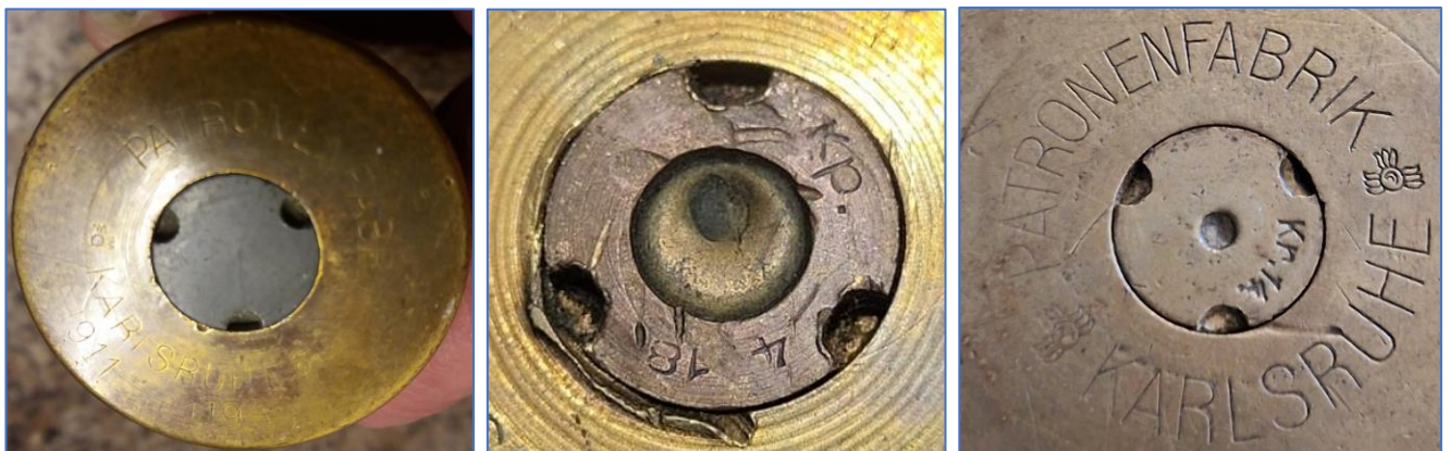
Figure 13: Left a solid 16 mm primer for export in a 1911 dated 37x94R44 shell case marked with Krupp shell case number 119 A ; middle the typical Krupp marked 16 mm primer with inner press-in primer, dated April 1918; right a very rare 1914 dated “Kr.” marked Krupp primer.
