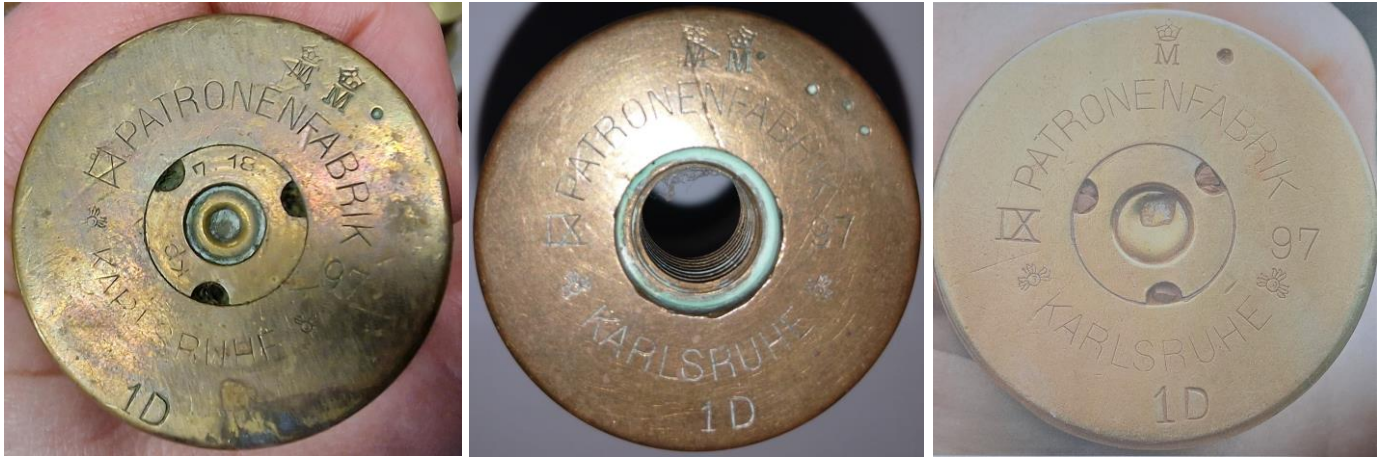
Figure 22: The earliest 37x94R44 shell cases existing with a Krupp 16 mm screw-in primer, dated September 1897. All 3 found examples are marked with "1D" and show signs of re-loading.
