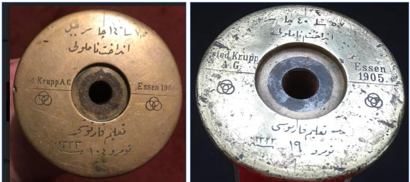
Figure 17: Sub-caliber training rounds for the 7,5 cm Krupp L/14 mountain gun (left) and the 5,7 cm Krupp L/40 navy gun (right).
