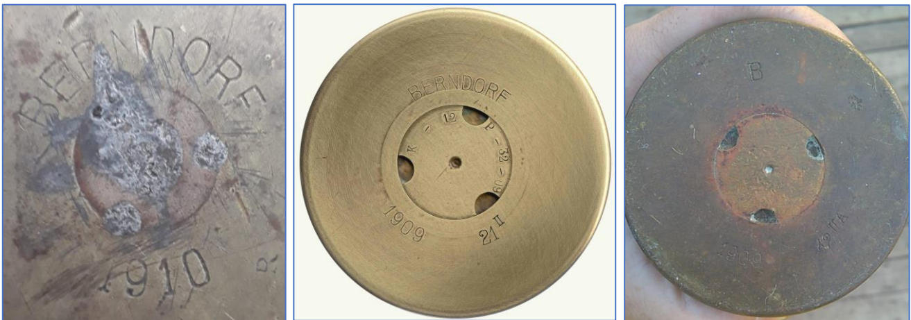
Figure 6: Examples of BMF manufacture. Left an example of a 1910 dated export case without Krupp shell case number, in the middle a 1909 dated shell case with Krupp shell case number 21 " (for Belgium), on the right a shell case dated 1909 with Krupp shell case number 42 "A for Brazil where only a letter “B” is stamped.
