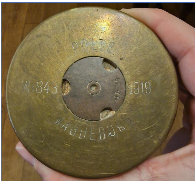
Figure 11: Head stamp of a 1919 dated Polte made 75x168R90 shell case for the Netherlands. The mark "Mh. 843" refers to Krupp "Metallhülse Nummer 843"; Krupp shell case number 843.
