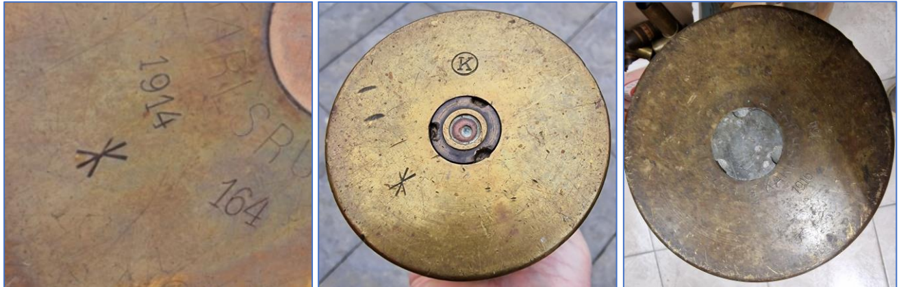
Figure 37: Left the unknown mark on shell case with Krupp number 164 (suspect Greece), middle the same mark found on a 47x158R64 shell case, right a shell case with zinc transport primer.
