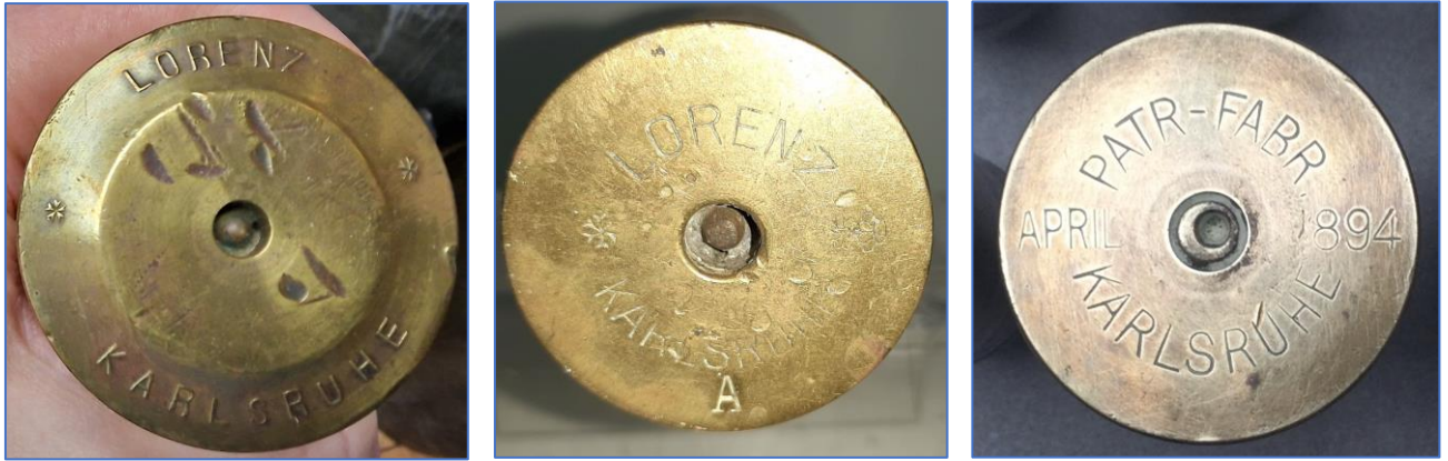
Figure 3a (1878-1894): Left is presumed the oldest example found with a 5-pointed “snow flake” (40x150R51, ~1878-1879); Middle is probably the oldest 37x94R44 shell case with a 6-pointed “snow flake” and a German army acceptance stamp (~1879-1881); Right a 37x94R44 dated 1894 without this mark. Note: My observations/interpretations for dating deviate slightly from Mellichamp 4 .
