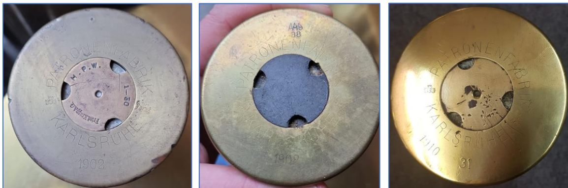
Figure 28: Left a Royal Netherlands East Indies army 1902 dated shell case, recognized by the primer (P.W. is for “Pyrotechnische Werkplaatsen”, “H” is unknown but suspected to mean “hervuld” meaning re-filled), middle a German 1908 dated shell case with zinc transport primer found in South-Africa, right a 1910 dated shell case with Krupp number 31.
