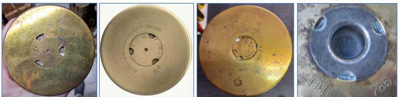
Figure 25: Left shell case number 21 for Turkey, then number 21 II for Belgium with Belgium made primer, then number 807 III A presumably for Romania, right a typical dummy transport primer found frequently in South-American counties like Argentina, Chile and Paraguay.
