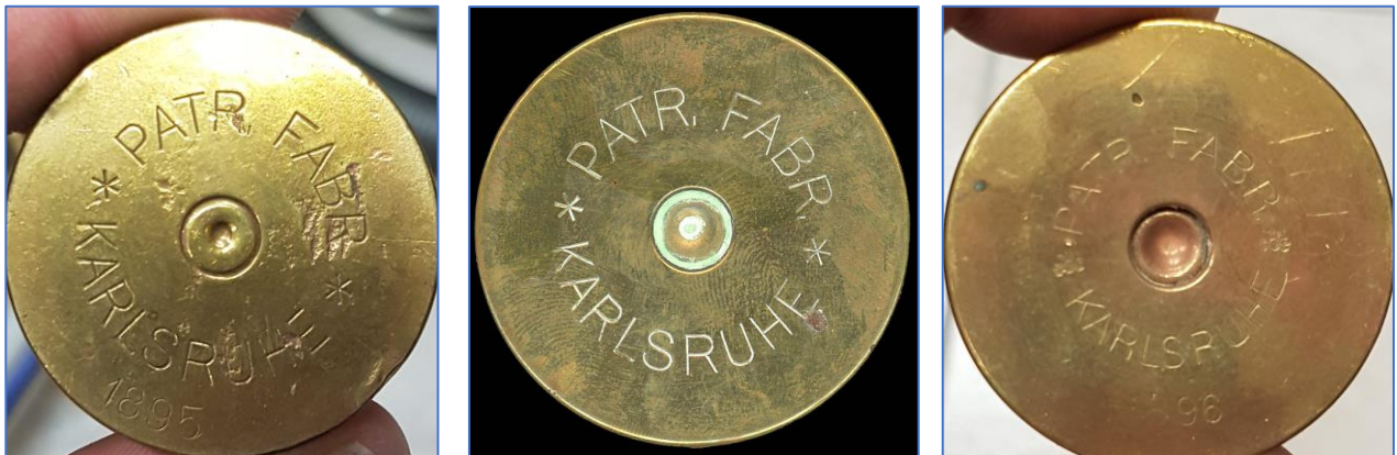
Figure 3b (1895-1896): Left the new style 6-pointed “snow flake”, only used in 1895, on a 37x94R44 dated 1895. Middle, an undated case with the same mark, but can be dated as 1895. Right a 37x94R44 with the introduction of the “flaming bomb” in 1896.
