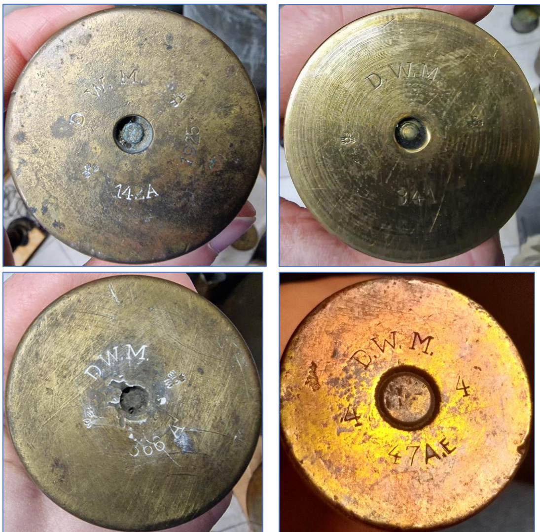
Figure 43: Four different head stamps for the unknown civil numbering system on DWM shell cases.
