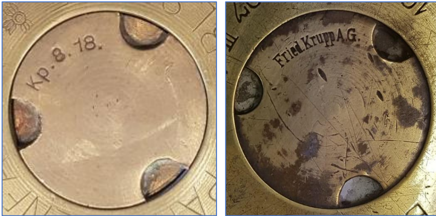
Figure 14: Left a 33 mm Krupp primer with less common late war stamp on shell cases; right a 33 mm Krupp primer with the more typical stamp.
