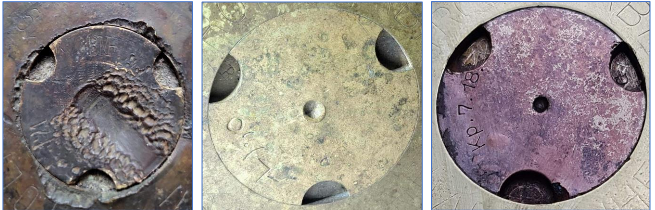
Figure 7: Left a primer marked “BMF”, middle a primer marked “B” (written in Ottoman “10,5 cm”) and right a 1918 Krupp primer marked “G”.
