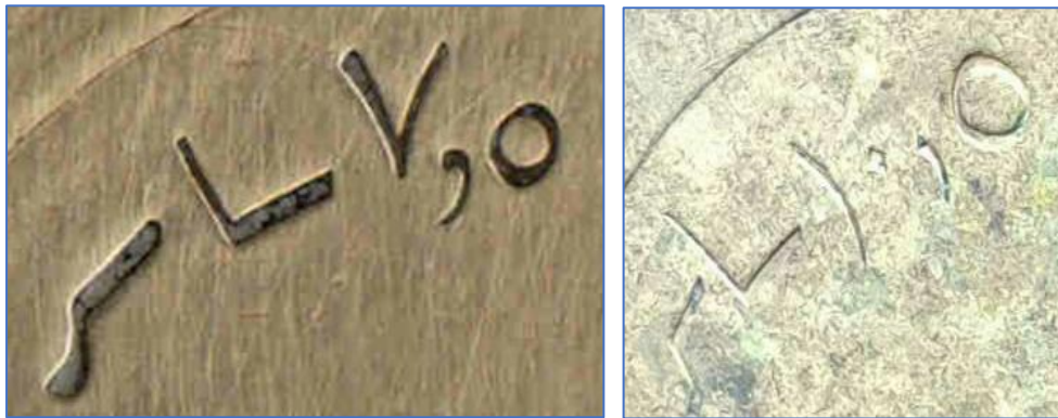
Figure 16: Ottoman writing on primers, left “7,5 cm” (۷,۵), right “10,5 cm” (۱۰,۵).
