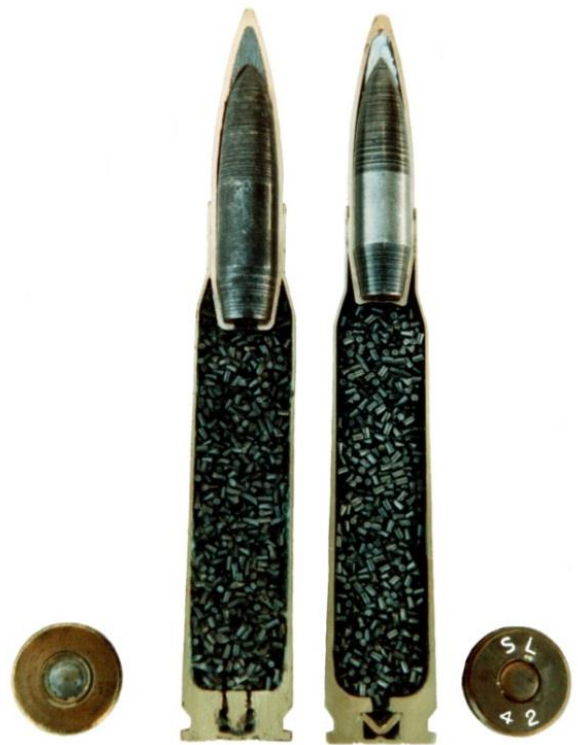
This photo illustrates the similarities between the Japanese 13.2x99mm AP cartridge on the left and the U.S. .50 caliber (12.7x99mm) M2 AP cartridge on the right. (Photo - George R. Masters)
