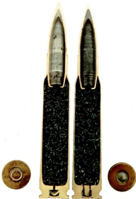
Armor Piercing examples are pictured. Note the white paint around the edges of the primers, circular primer crimps, and steel cores. The round on the left has a Boxer primer, while the round depicted on the right has a two-hole Berdan primer. (Photo - George R. Masters)
