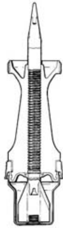
Cross-section drawing of projectile assembly for 120 mm APFSDS-T L23 produced by RO Defence (2000)
