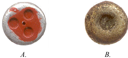
Fig. 9-18. Mark II short-delay fuse cup ends. (A.) 3-hole cup with red igniter. The cartridge with this cup is shown above in Figure 9-17. (B.) 1-hole cup, from a test failure round. 3x actual size.
